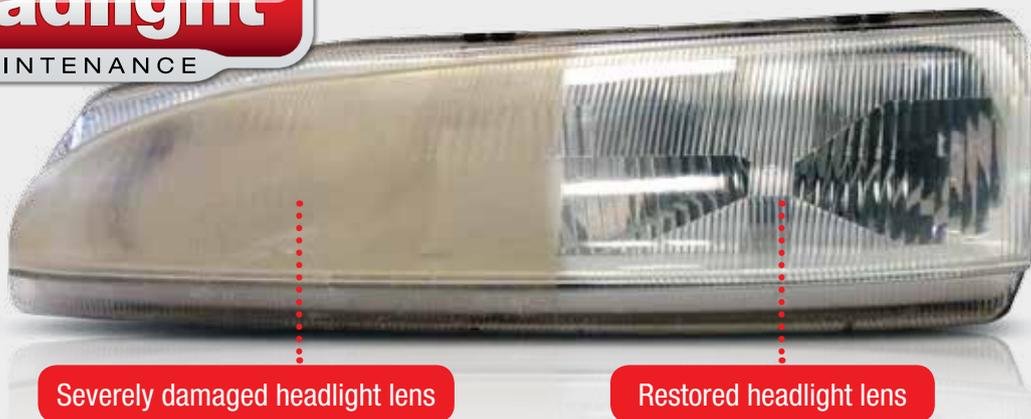
Severely damaged headlight lens
